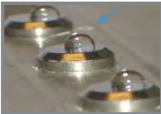
Droplets “bead up” on properly conditioned pedestals
